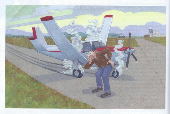
THE BRAKES ON SMALL AIRPLANES have three functions: to decelerate the airplane after landing; to hold the airplane whenever it needs to be motionless; and to assist with ground maneuvers. The first may be what comes to mind for nonpilots accustomed to hard braking and roaring thrust reversers during an airliner landing, but it should be avoided by the average pilot.
